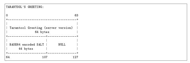
The server instance begins the dialogue by sending a fixed-size (128-byte) text greeting to the client. The greeting always contains two 64-byte lines of ASCII text, each line ending with a newline character ("\n"). The first line contains the instance version and protocol type. The second line contains up to 44 bytes of base64-encoded random string, to use in the authentication packet, and ends with up to 23 spaces.
