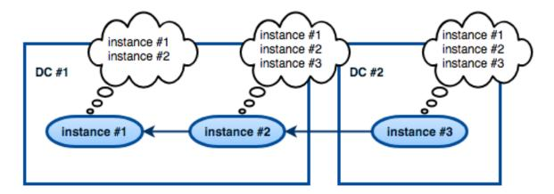
We have a chain of three instances. Instance #1 contains entries for instances #1 and #2 in its \_cluster space. Instances #2 and #3 contain entries for instances #1, #2 and #3 in their \_cluster spaces.
