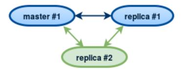
To add a second **replica** instance to the **master-replica** set from our *bootstrapping example*, we need an analog of the instance file that we created for the first replica in that set:
