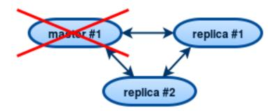
In a master-replica set, if a master disappears, error messages appear on the replicas stating that the connection is lost:
