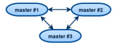
The failover benefit in this case is still present, and the load-balancing benefit is enhanced, because any instance can handle both read and write requests. Meanwhile, for multi-master configurations, it is necessary to understand the **replication guarantees** provided by the asynchronous protocol that Tarantool implements.
