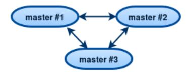
You then can decide where to locate instances of the mesh – within the same data center, or spread across a few data centers. Tarantool will automatically ensure that each row is applied only once on each instance. To remove a degraded instance from a mesh, simply change replication configuration parameter.
