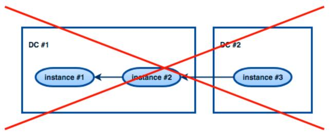
The problem with a cascading replica set is that some instances have no connection to other instances and may not receive changes from them. One essential change that must be propagated across all instances in a replica set is an entry in box.space.\_cluster system space with replica set UUID. Without knowing a replica set UUID, a master refuses to accept connections from such instances when replication topology changes. Here is how this can happen:
