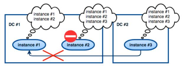
Now instance #2 is faulty. Instance #3 tries connecting to instance #1 as its new master, but the master refuses the connection since it has no entry for instance #3.
