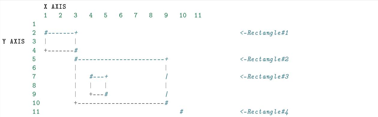
The rectangles are defined according to this scheme: {X-axis coordinate of top left, Y-axis coordinate of top left, X-axis coordinate of bottom right, Y-axis coordinate of bottom right} – or more succinctly:  $\{x_1, y_1, x_2, y_2\}$ . So in the picture ... Rectangle#1 starts at position 1 on the X axis and position 2 on
